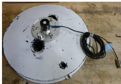
Licor LI-190SA ambient sensor with levelling fixture.
