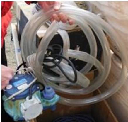
Figure 4. The peristaltic pump used to pump the water from the funnel of the sediment trap upon retrieval from lake (only needed if the funnel does not drain properly).
