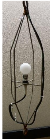
Licor LI-193SA UW sensor with lowering frame.
