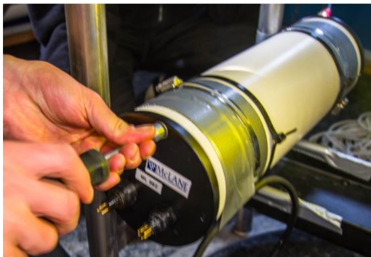
Figure 10a. Removal of screws from the sediment trap housing USING A NUT DRIVER.
