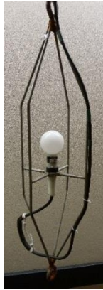
Licor LI-193SA UW sensor with lowering frame.
