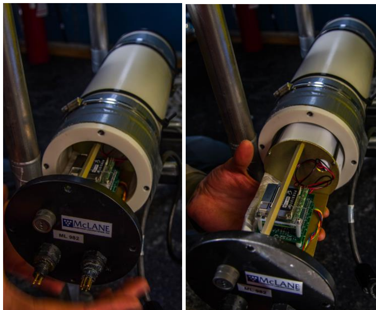
Figure 10b. Removal of the controller with battery pack assembly from the sediment trap housing.
