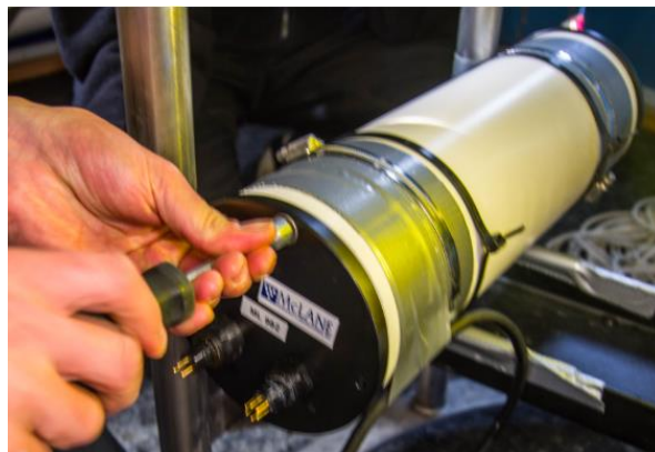
Figure 16b. ONLY USE A NUT DRIVER to tighten the screws into the housing.
