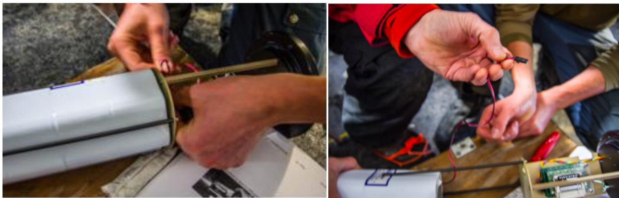
Figure 13. Unplugging of battery pack wires from the electronics panel.
