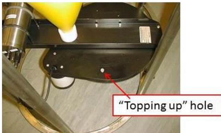
Figure 8. “Topping-up” hole used to fill bottles after they have been inserted into carousel.
