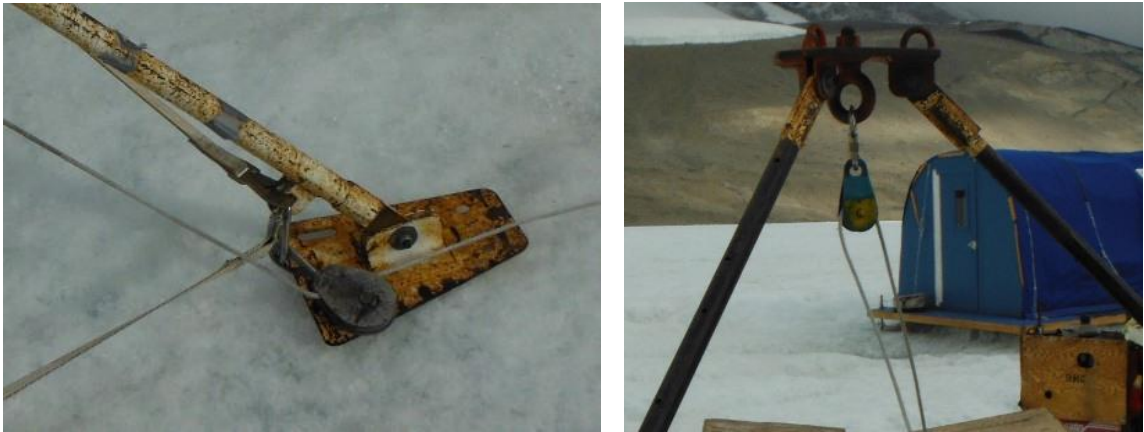
Figure 3. Location of pulleys on the tripod.
