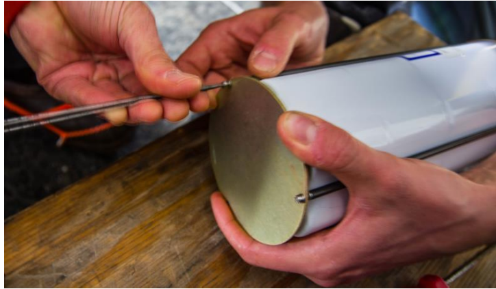
Figure 12. Removal of the metal cover from the back of the assembly.
