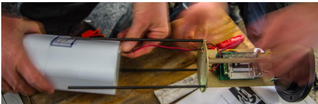
Figure 13b. Removal of Alkaline battery pack from assembly (unplug wires first – this photo was a demonstration before the wires were unplugged).
