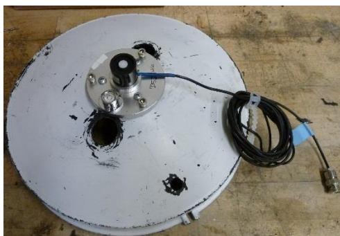
Licor LI-190SA ambient sensor with levelling fixture.
