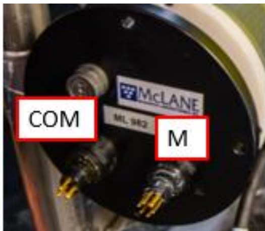
Figure 17. Connection ports on the controller with battery pack assembly cover for connection to the computer (“COM”) and motor (“M”).
