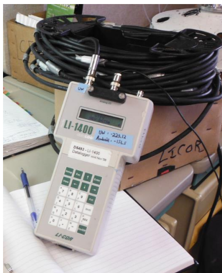
Licor LI-1400 Data Logger with 30m underwater cable.
