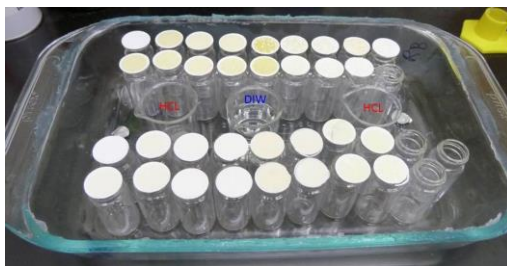
Figure 1. Acidification of filters.
