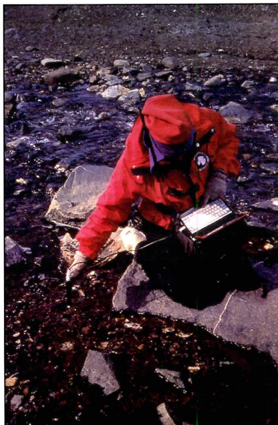
Scientist measures the spectral reflectance of microbial mat in a stream.
