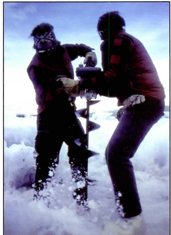
A Jiffy drill is used to make a collection hole in an ice-covered lake.
