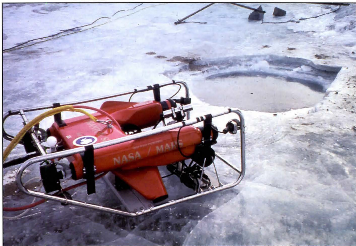
A remotely-operated vehicle (ROV) used to explore the under-ice environment of an ice-covered lake. This particular ROV had a range of 150 m.
