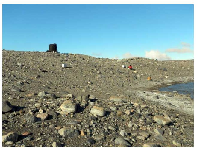
The south-facing hillslope of Many Glaciers Pond showing the location of the Pulse-Press Project. The large black structure on the ridge is a 1000 gallon holding tank. White boxes are insulated instrument power arrays and data storage modules (Photo: MCM LTER).
