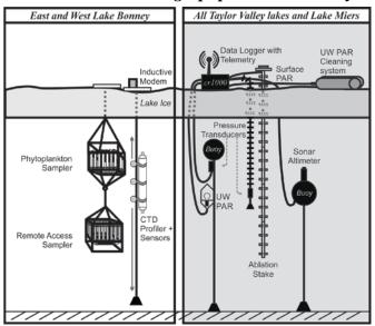
Fig. 1. Schematic showing autonomous sampling (left) and monitoring (right) equipment deployed in MCM LTER lakes
