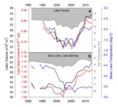
Fig. 3. Decadal changes in lake volume, heat content, ice thickness (gray fill), and volume-weighted mean temperature for (a) lake Frxyell and (b) East Lobe of Lake Bonney.
