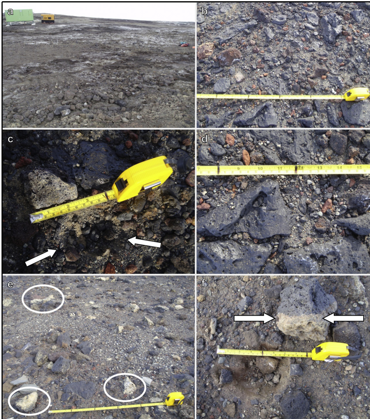
Fig. 1. Examples of the Desert Pavement Recovery Assessment (DPRA) criteria I–V (Tables 1 and 2). a) Embeddedness of surface clasts, DPRA rating 1, clearly disturbed; b) embeddedness of surface clasts, DPRA rating 4, undisturbed; c) impressions of removed clasts, DPRA rating 0, highly disturbed (arrows indicate impression); d) degree of clast weathering, DPRA rating 2, moderately weathered (varnish and pitting); e) % overturned clasts (salt side up, circles indicate overturns), DPRA rating 2, moderately disturbed, 20–50% clasts overturned; f) salt on underside of clasts, as part of “10 cobble” test.
