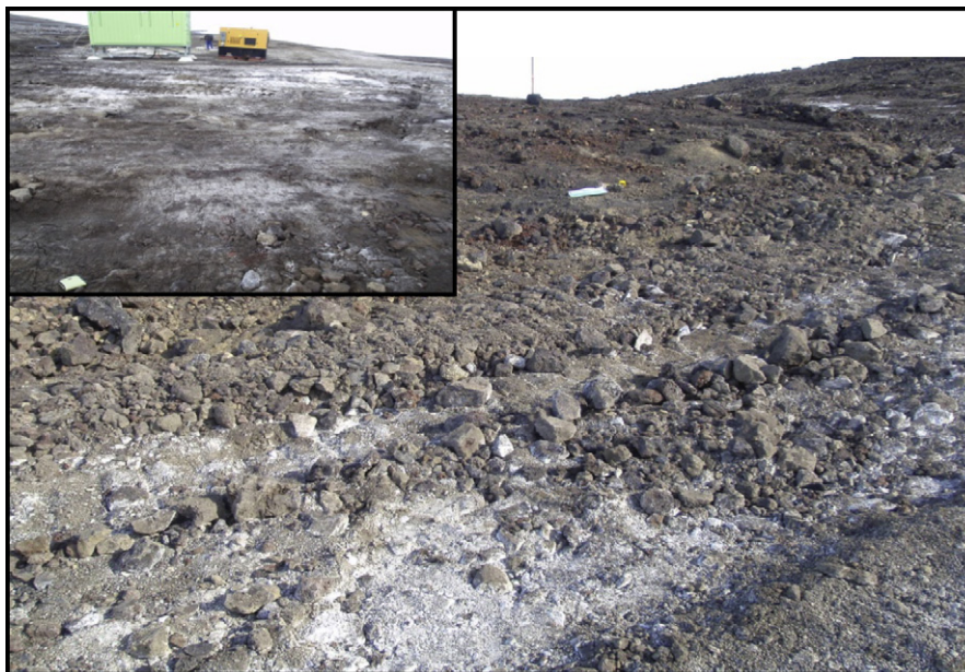
Fig. 6. Crater Hill site A. Mean Recovery Index = 23%. Note lack of clast embeddedness, desert pavement armouring, high% overturned clasts, and accumulation of salt on the newly disturbed surface.
