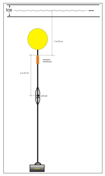
**Fig. 7:** Buoy at East Lobe of Lake Bonney. (not to scale)
