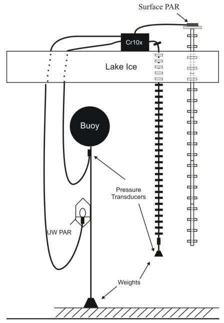
**Fig.1**: Lake cross-section showing buoy, data logger, position of deployed sensors and ablation stake.
