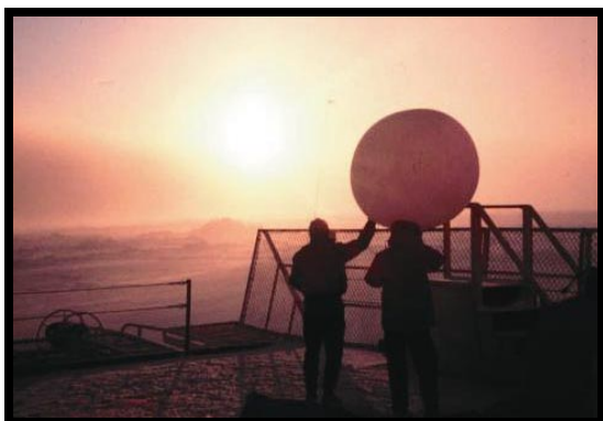
Launching a radiosonde off the helicopter deck of the R.V. Nathaniel B. Palmer, Ross Sea, August 1995.
